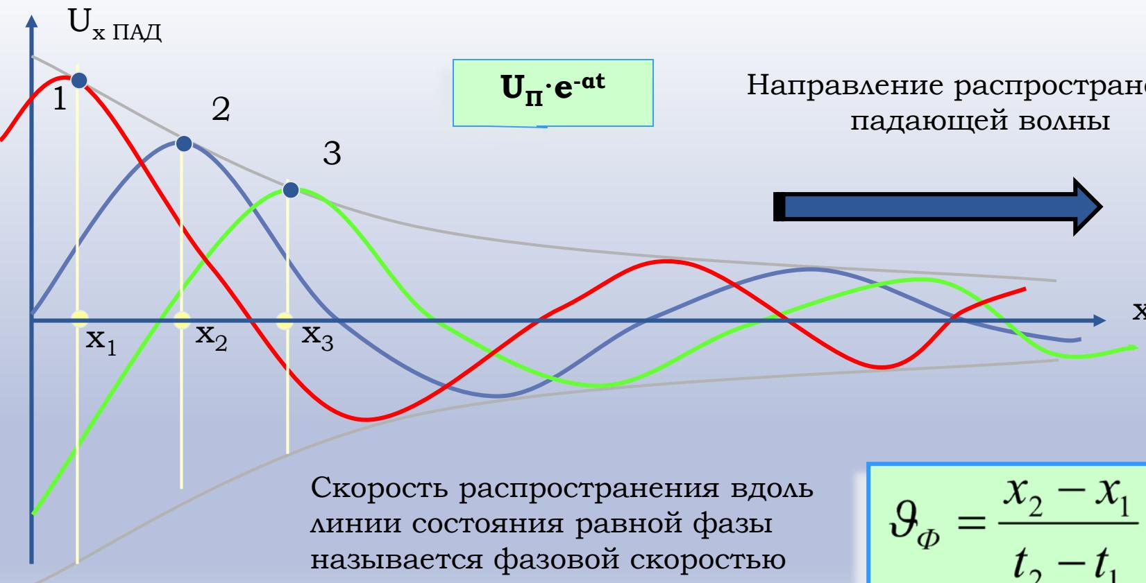
$$U_x(t) = U_{\Pi} \cdot e^{-\alpha t} \sin(\omega t - \beta x) + \underline{U_O \cdot e^{\alpha t} \sin(\omega t + \beta x)}$$
