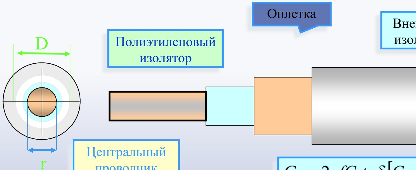
$$R_0 = 8,33\sqrt{f} \left( \frac{1}{d} + \frac{1}{D} \right) \rightarrow [O\mu\text{m}/\text{m}]$$
