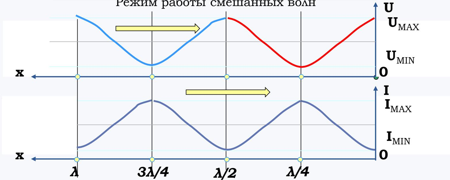
$$k_{BB} = \left| \frac{U_{\min}}{U_{\max}} \right| = \left| \frac{U_{\text{ПР}} - U_{\text{ОБР}}}{U_{\text{ПР}} + U_{\text{ОБР}}} \right| = \left| \frac{I_{\min}}{I_{\max}} \right|$$
